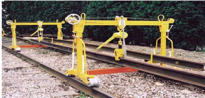
The Ironmen were being operated down a gradient which was up to 1 in 40, with the load for each pair being just short of 1 tonne. The rail head was contaminated with leaves and it was raining heavily at the time.
