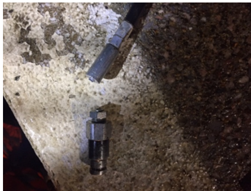
Photograph showing hose connector snapped.
